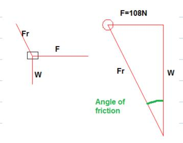
From CAD, weight force Fn = 216.0005N So mass = 216.0005/9.81 =22.0184 kg
