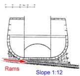
Slope is measured as a rise of 1 for every 12 along the ramp. (12 is hypotenuse, not the horizontal)
